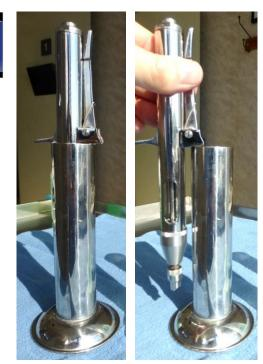
The problem with the steel cylinder was that its **opacity** made it difficult to determine the depth of the MadaCide. One could try to see how much of the MadaJet got wet with immersion, but the depth could decrease unnoticed as the day wore on.
